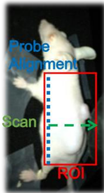
Figure 2.3: ncDCT mouse tumor data acquisition. Illustration of the mouse orientation with respect to ROI, noncontact probe alignment, and scan direction.
